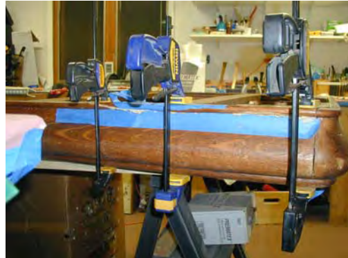
Epoxy wood filler/glue applied on top of hide glue and mating ends clamped
