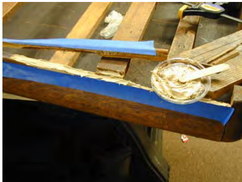
Epoxy wood filler/glue applied on top of hide glue and mating ends clamped
